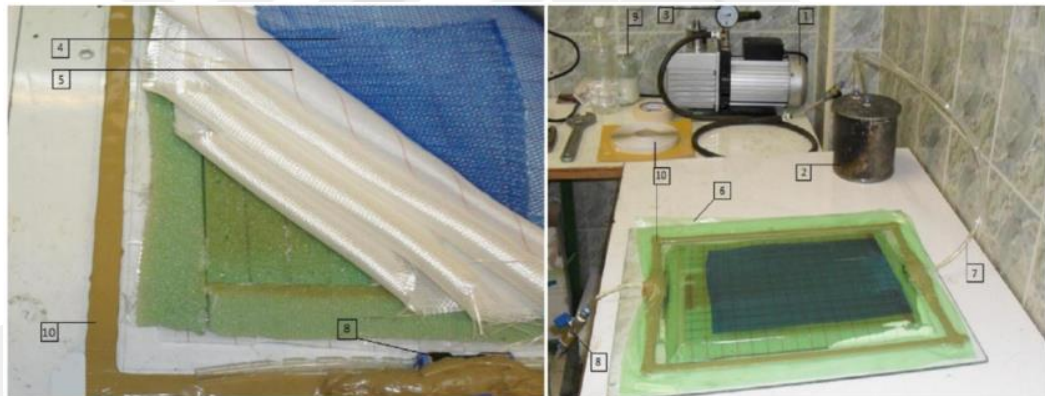
Figure 1.8 Detail of VARTM Process. 1- Vacuum Pump, 2- Safety Tank, 3- Indicator, 4- Distribution Layer, 5- Dacron Peel Ply, 6- Vacuum Bag, 7- Resin Transfer Tube, 8- Valves and Joints, 9- Release Wax, 10- Seal Paste [40]
