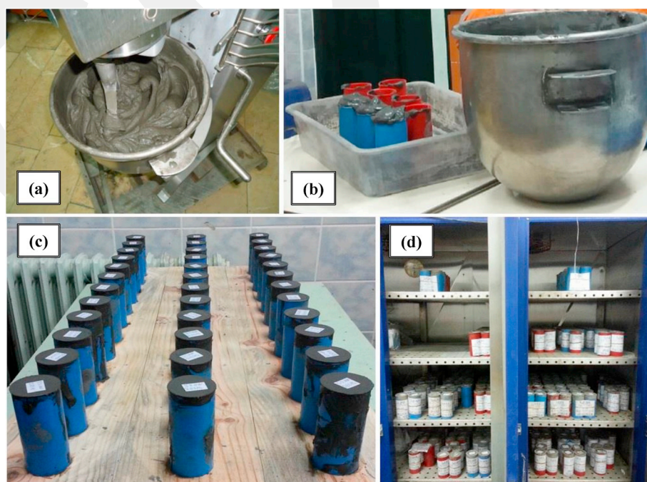
Fig. 4. Preparation of CPBs: mixing (a), casting (b), draining (c) and curing (d).
