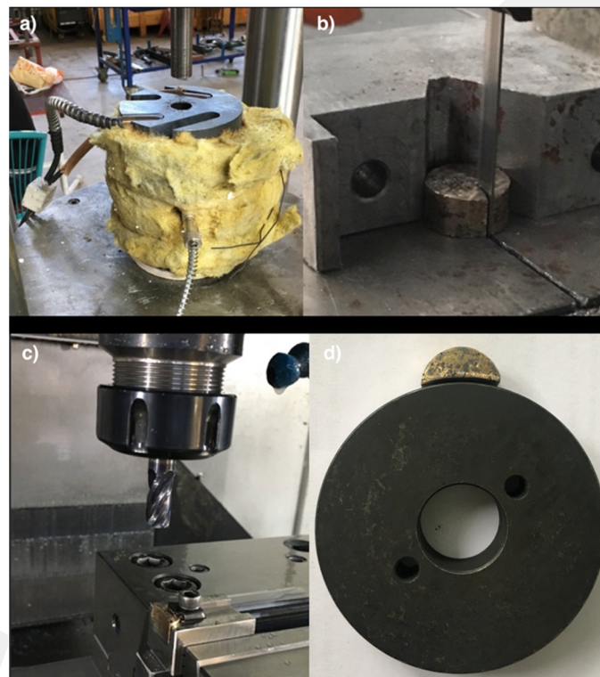
Figure 1. Composite materials: (a) production, (b,c) preparation for wear tests, and (d) composite and abrasive disc before wear test.
