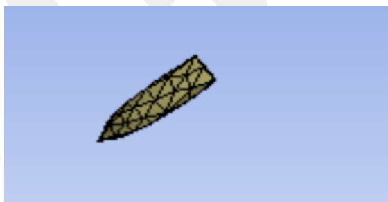
Figure 3.3 Meshed visual of 7.62 mm projectile
