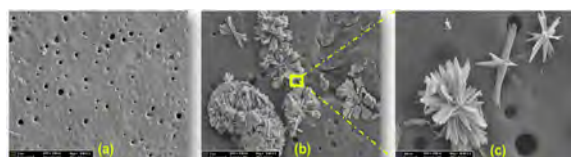
Figure 3. Schematic illustration showing the Scanning electron microscopic images of (a) PSF membrane, (b) Gd 2 O 3 /PSF membrane, and high-magnification of flower shape.
