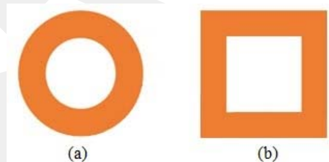
Fig. 1. Conventional coil structures: a) circular shaped coil and b) square shaped coil.
