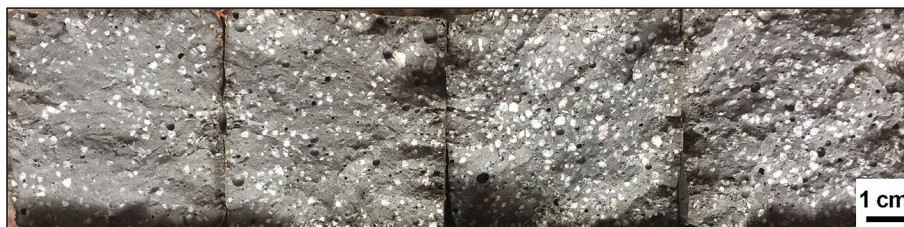
Fig. 12. Broken specimens obtained using pre-wetted EP.
