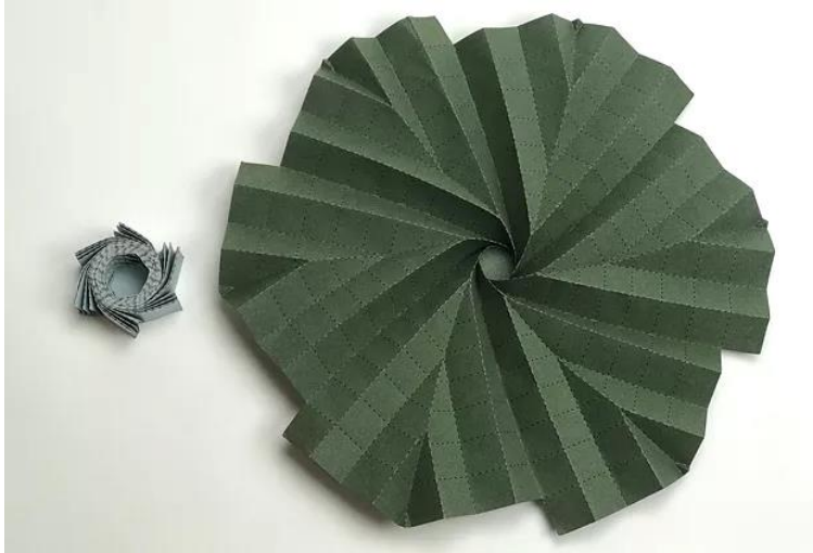
Figure 2.19 Flasher model that can be stored in the compact central volume (Hummel, 2020)
