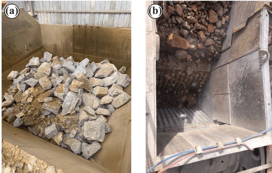
Fig. 1. Illustration of choke feeding intensity for an industrial jaw crusher a) Fully loaded feeding bunker b) Uncontrolled choke feeding intensity in the crushing chamber.
