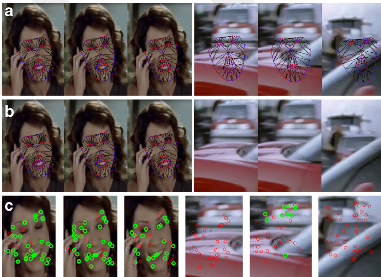
Fig. 2 a Six consecutive frames from a movie is shown. Face Tracker continues to track the landmarks although there is a sudden scene-cut. b The proposed SURF-features based method helps to stop face tracking at a scene cut. c Green circles denote matching SURF features between the current frame and the previous frame from left, red circles denote features that have not matched. There are no matching SURF features at the fourth frame from left, indicating a scene cut
