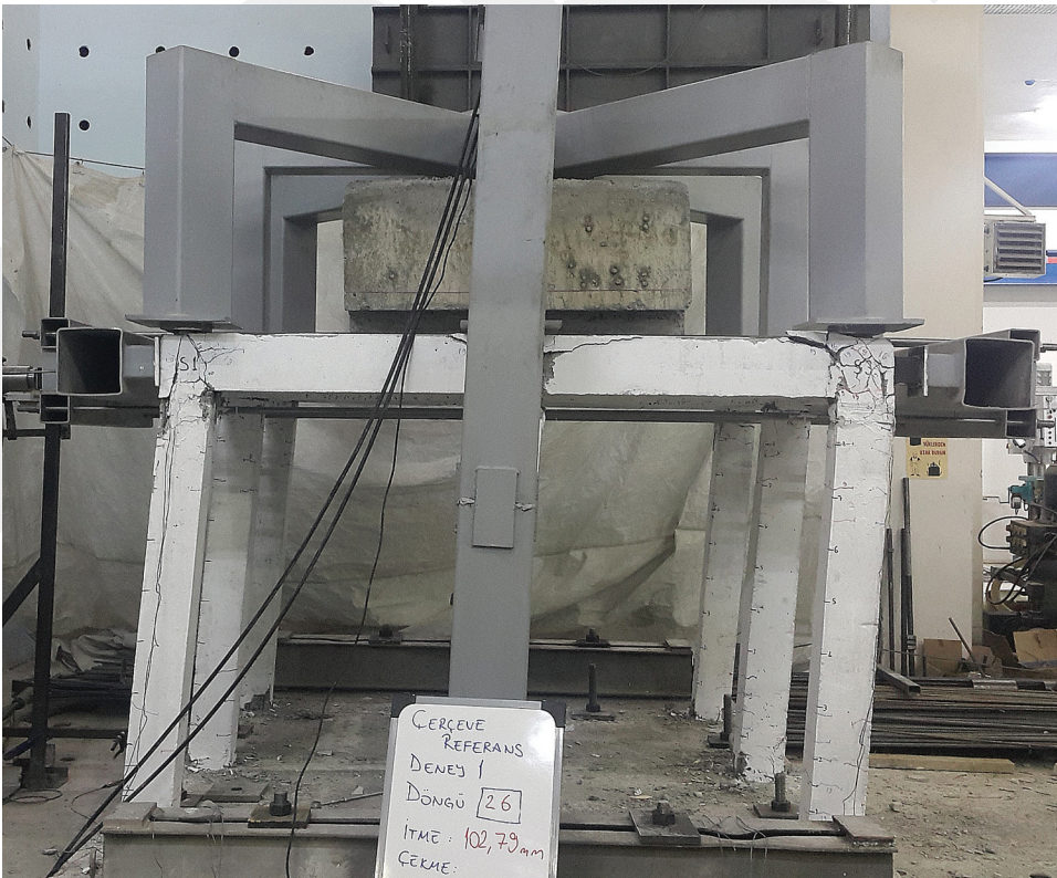
Figure 7. The reference frame at the end of the test.
