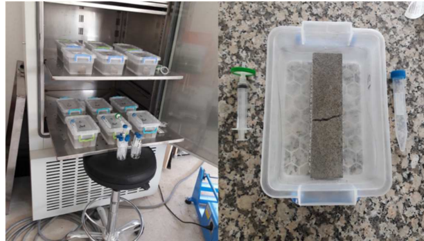
Figure 1. Experimental Setup for Nutrient Leaching Tests.
