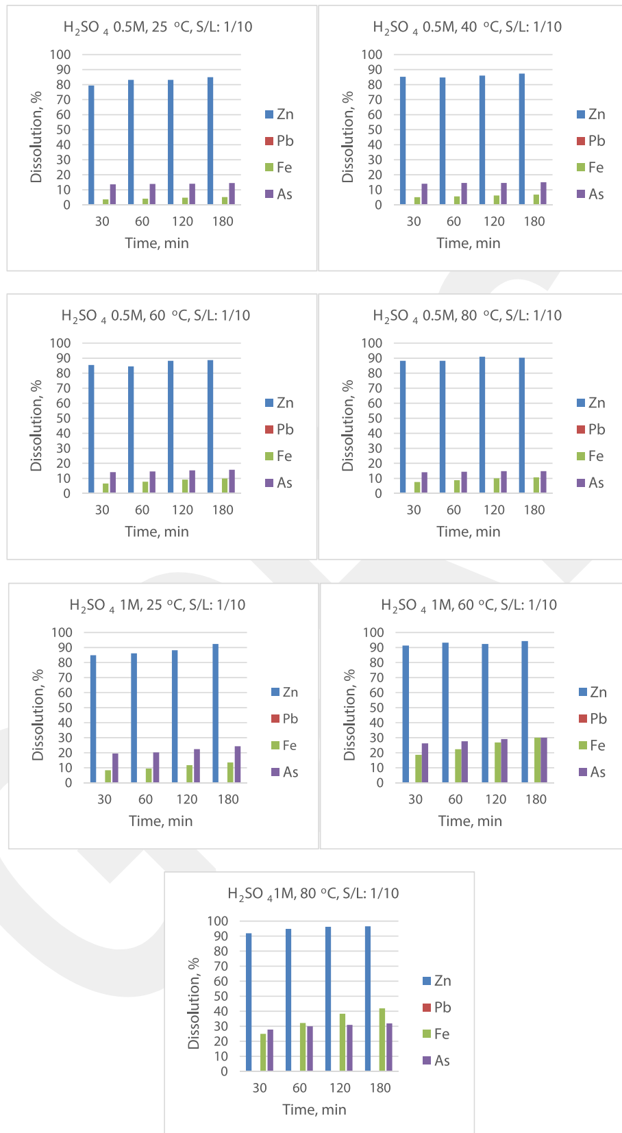
Fig. 3. Effect of temperature on dissolution at 0.5 M and 1 M sulfuric acid concentration.
