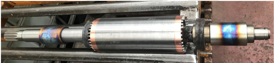
Figure 6.12 Finished rotor after bearings are inserted
