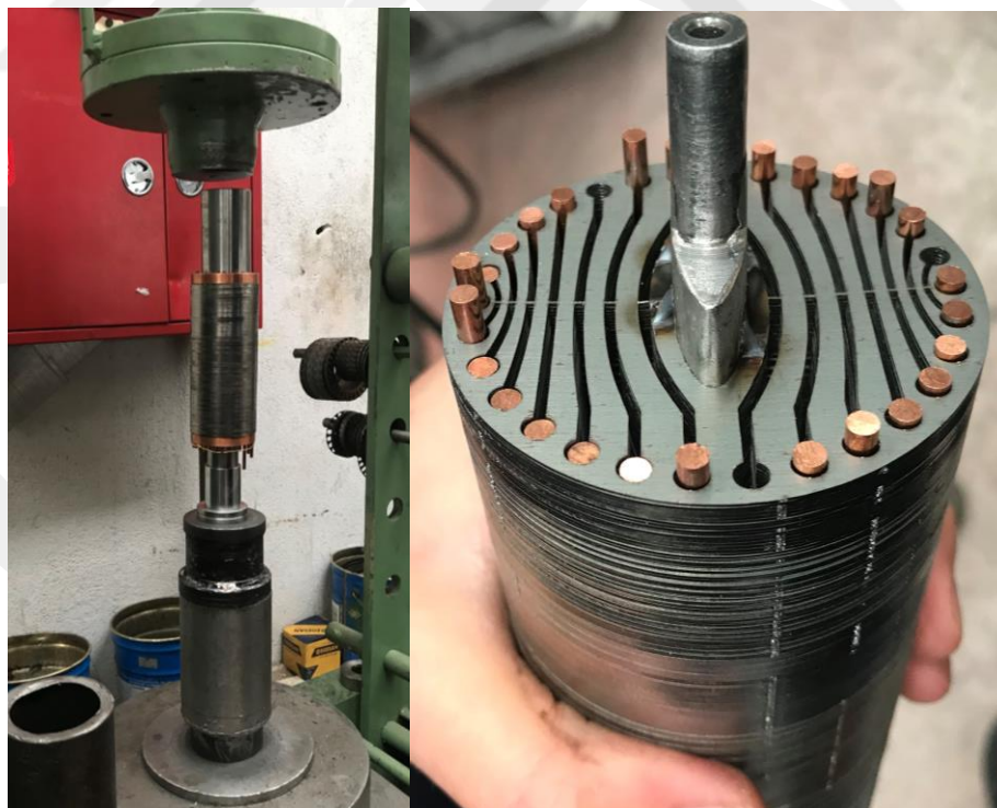
Figure 6.8 (a) Rotor stack pressed together and (b) welded to the shaft
