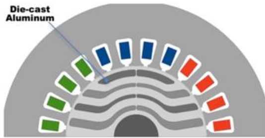
Figure 2.9 Cross section of the motor [39]
