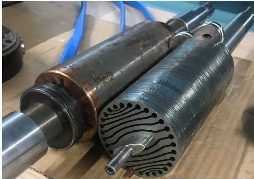
Figure 6.7 Stacked rotor laminations onto the oval shaft
