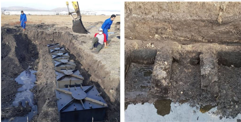
Fig. 6 Undisturbed sampling process for organic soil
