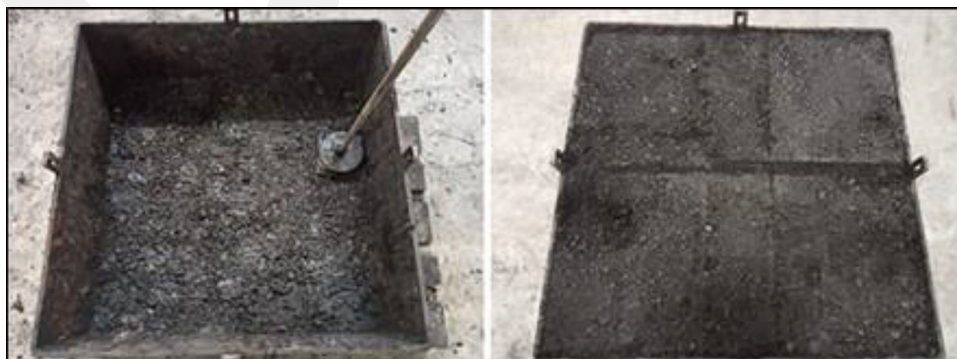
Fig. 7 Compaction of disturbed organic soil
