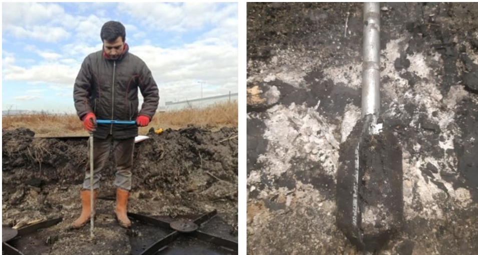
Fig. 14 Implementation of the Vane shear test in the site and laboratory
