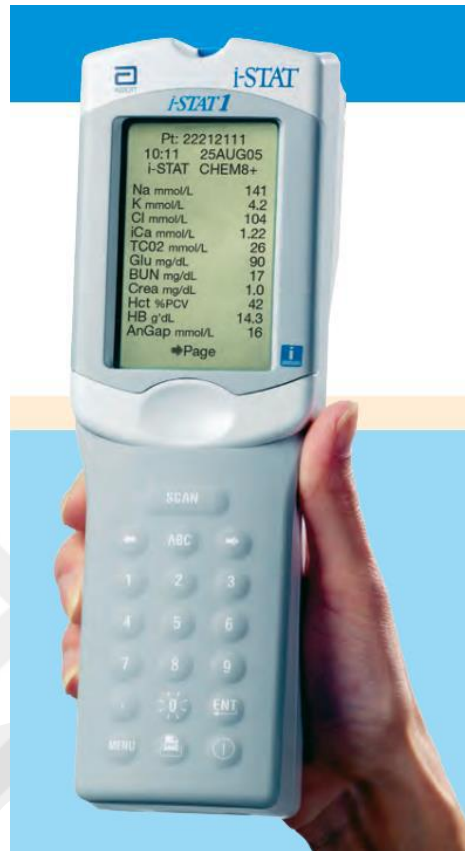
Figure 2.1.2.1.1 An example of electrochemical biosensor called i-STAT [42]. The device can analyze blood samples in a few minutes.
