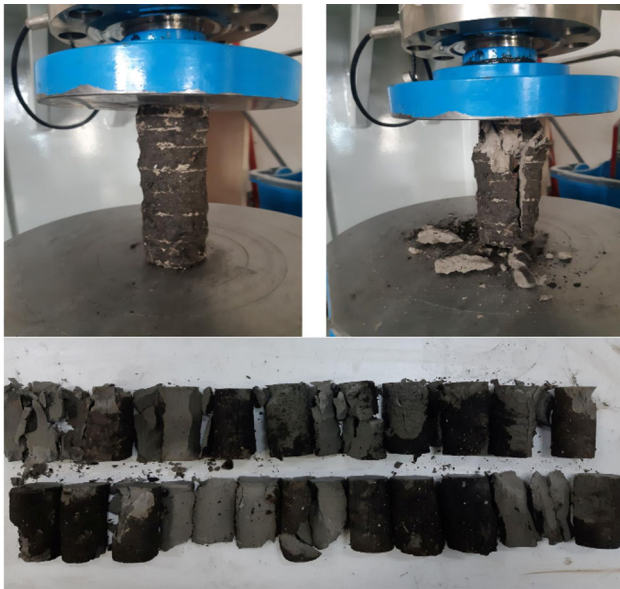
Fig. 18 Uniaxial compressive strength test on excavated soilcrete samples
