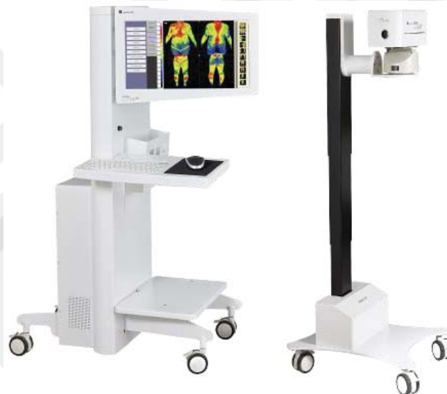
Figure 2.16 Medicore IRIS-XP medical infrared thermography system
