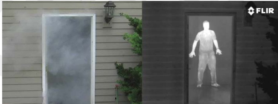
Figure 2.4 How thermal imaging cameras can see through smoke
