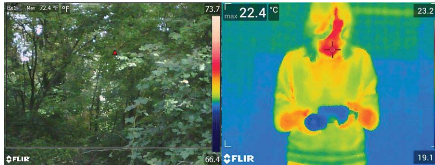
Figure 2.5 Thermal reflection from glass
