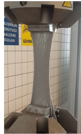
Figure 4. Deformed geotextile specimen
