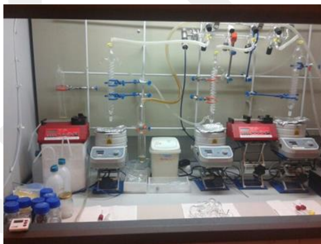
Figure 2.1.2. 1 Nanocrystal synthesis system composes of shlenk-line, heater, vacuum pump, vacuum gauge, condenser, clips and temperature probe.
