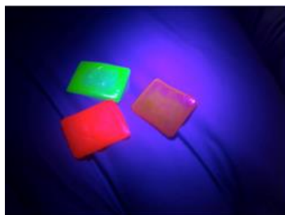
Figure 3.1.2. 5 Free-standing sheets of CdSe/ZnS quantum dots under UV light. Reprinted with permission from [27]. Copyright 2016 IOP Publishing.
