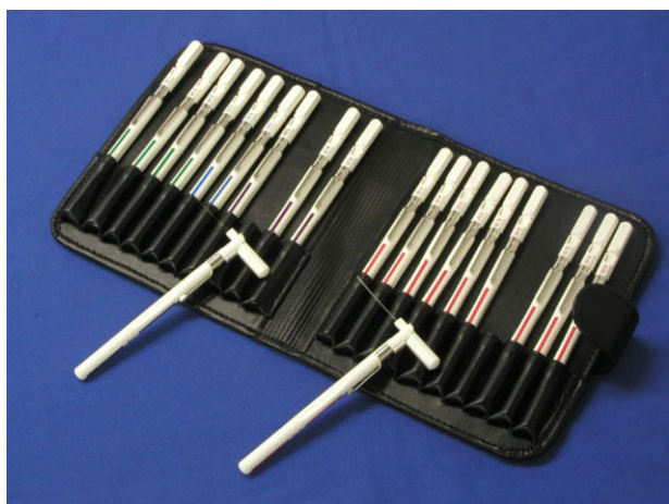
FIG. 1. TOUCH SENSATION TEST KIT CONSISTING OF 20 SEMMES-WEINSTEIN MONOFILAMENTS
