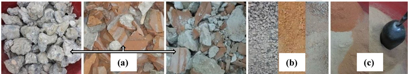
Fig. 1 Main components of CDW (a) and size reduction operations (crushing (b), grinding and mixing (c))
