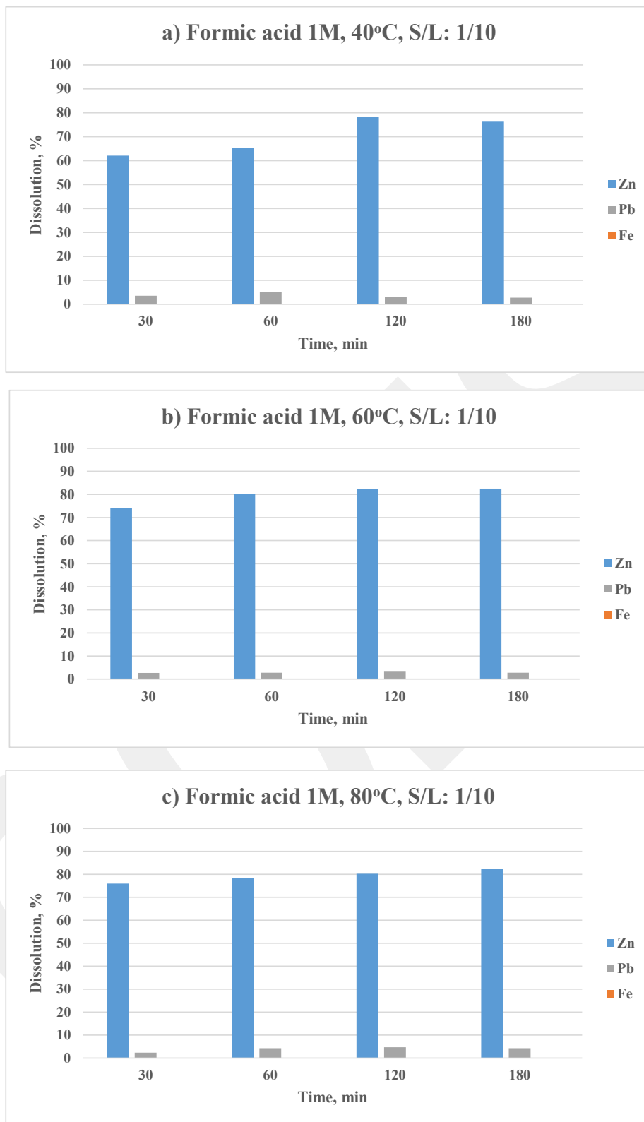
Fig. 11. The effect of temperature and leaching time on the dissolution of metals from the flotation tailing using formic acid.
