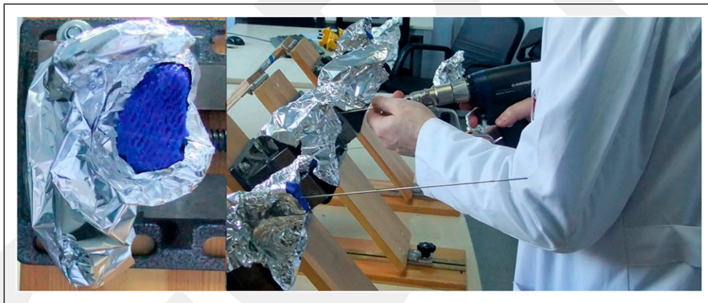
Figure 3. (Left) Scapula model covered by aluminum foil, mounted on the fixture, (Right) Experiment setup, surgeon inserting the guide pin with the freehand method.
