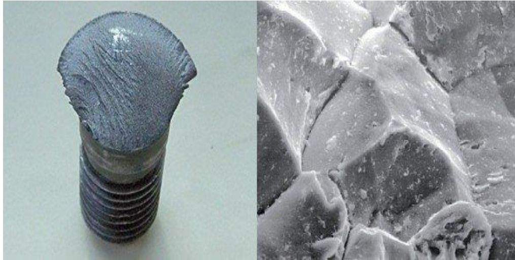
Figure 1.8 Cracks due to the hydrogen embrittlement [61].
