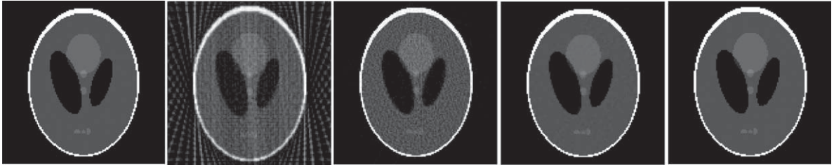
Fig. 1. Reconstructed Images. (from left to right): Original image, FBP, ART, ART + TV, (ART + TV)NLM.
