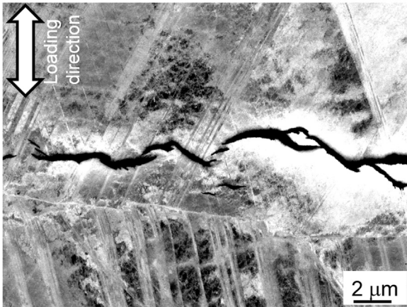
Fig. 10. ECC image showing curved-crack cross deformation twin plates in the fractured specimen pre-charged with hydrogen.
