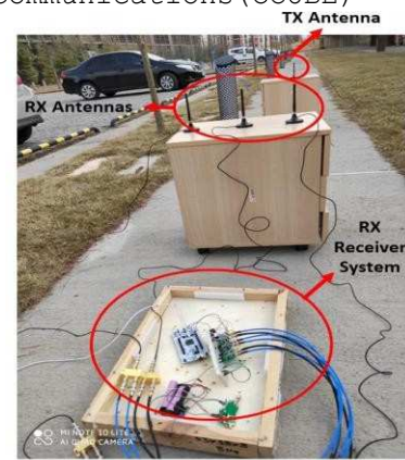
Fig. 8. Photo of the receiver system captured during experiments with the receiver antennas connected to the receiver system and the transmitter antenna on the same horizontal plane in open space.
