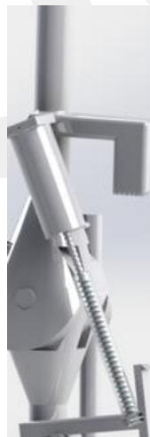
Figure 3.1.4.1 Ball-screw mechanism, motor and elastic element for stair-climbing function
