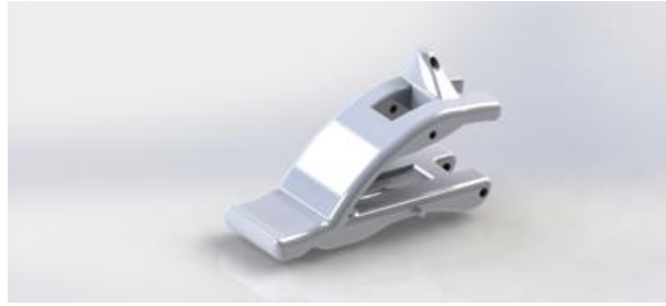
Figure 3.1.6.2 CAD design of catapult like ankle-foot compartment of prosthesis
