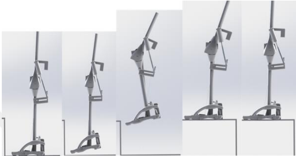
Figure 3.1.4.2 Stair climbing function of conceptual design
