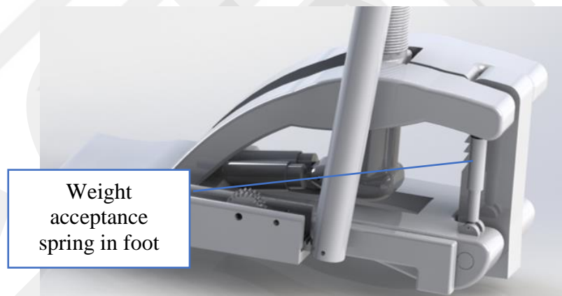
Figure 4.1.4.1 Weight acceptance spring in catapult mechanism
