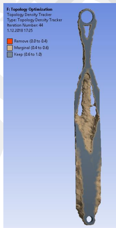
Figure 5.1.6.14 Topology optimization of the modified connection part.
