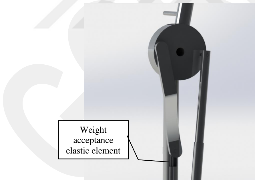
Figure 4.1.1.1 Weight acceptance elastic element
