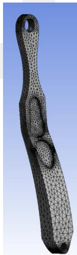
Figure 5.1.6.16 Mesh of the modified connection part.
