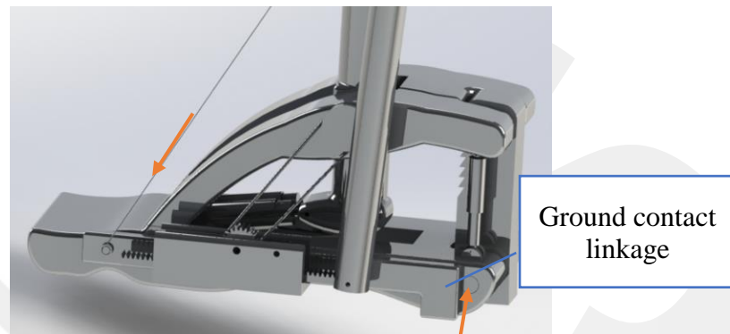
Figure 4.2.1.4 Engage-disengage mechanism on foot compartment
