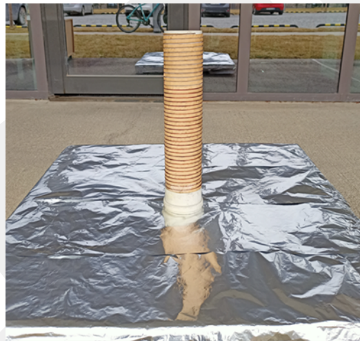
Figure 18. The designed system with the prototype antenna placed on a square-shaped ground plane with a 1-m side length.
