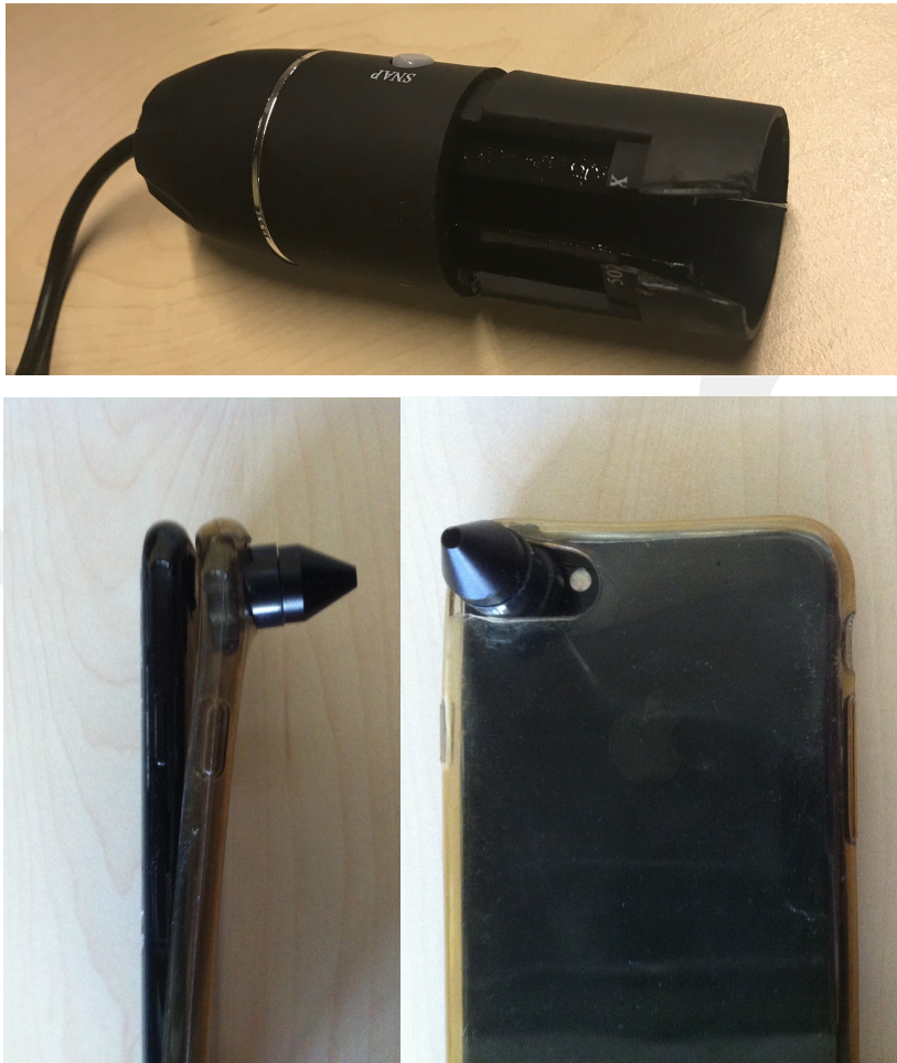
Figure 3.2.3.1 Lens is attached to the rear camera of our smartphone in order to provide an optic zoom to the camera. Lens is fixed with a silicon phone case.
