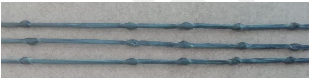
Figure 1. Knotted carbon-based bars used in the production of the new generation blade.
