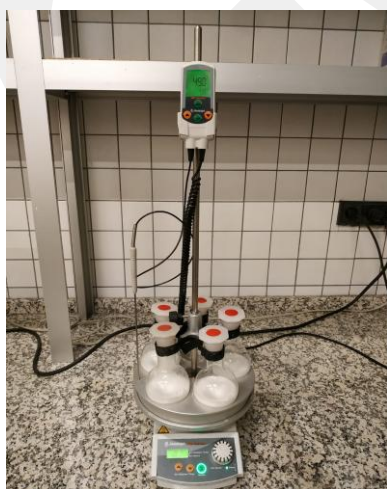
Figure 2.1 Hydrolysis set up
