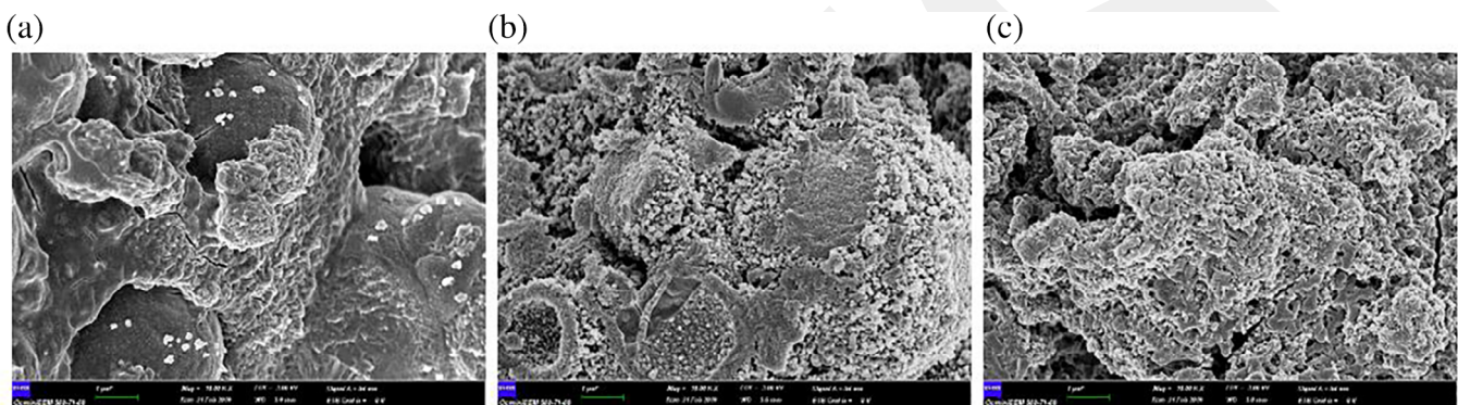
FIGURE 7 Field-emission scanning electron microscopy (FESEM) images of geopolymer samples after 24 hr 75°C heat curing (a) without nanoparticle (b) containing 2% NS (c) containing 2% NC
