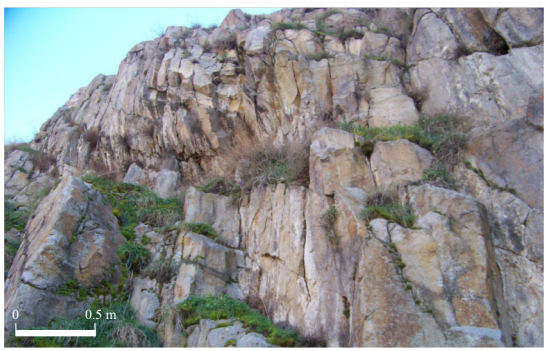
Fig. 6 Highly-jointed andesite at 4th (S4) location
