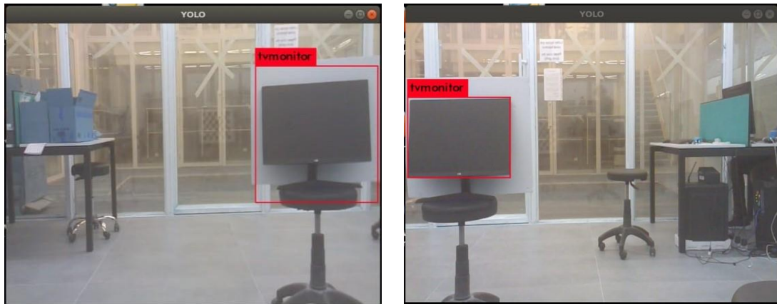
Figure 5.7 Detection of the object in a straight direction with a) Left drone and b) right drone
