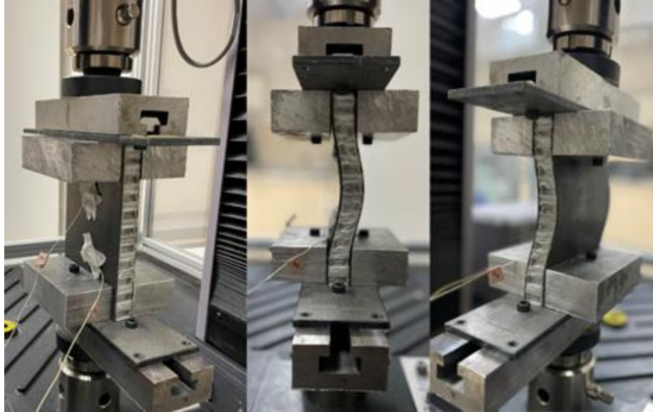
Figure 3.2 Position of the AE sensors and the deformed specimen after the compression test.
