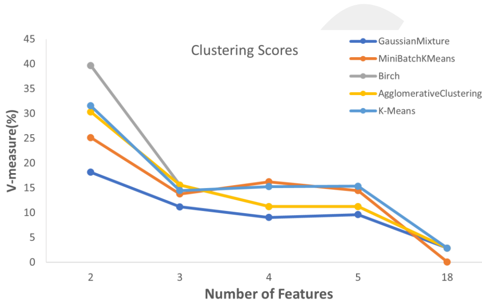
Figure 3.7 Comparison of clustering scores (V-measure) for various algorithms across different numbers of features under the peak frequency target.
