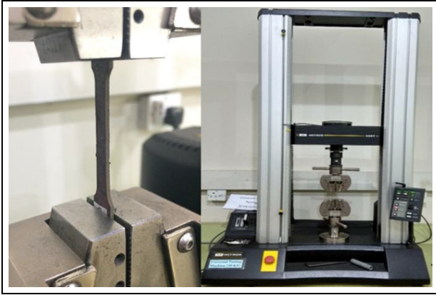
Figure 1. Experimental setup for tensile testing.
