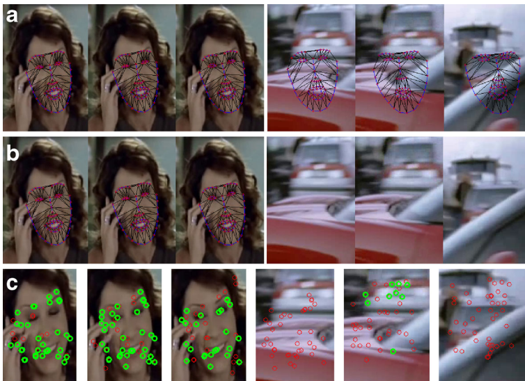
Fig. 2 a Six consecutive frames from a movie is shown. Face Tracker continues to track the landmarks although there is a sudden scene-cut. b The proposed SURF-features based method helps to stop face tracking at a scene cut. c Green circles denote matching SURF features between the current frame and the previous frame, red circles denote features that have not matched. There are no matching SURF features at the fourth frame from left, indicating a scene cut
