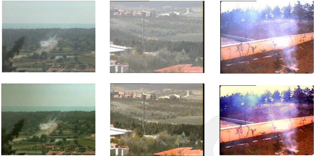
Figure 3.14. First row demonstrates three original dataset images in the smoke/non-smoke database, and the second row indicates their dehazed counterparts.
