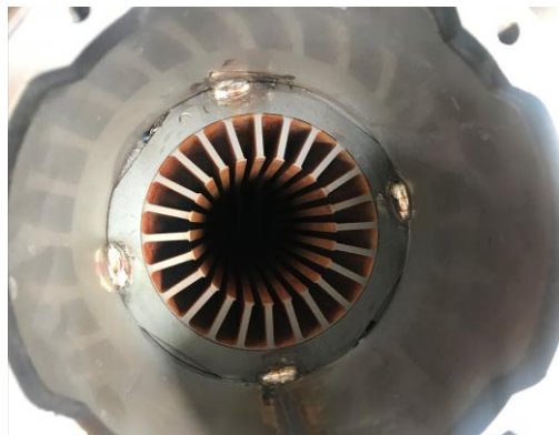
Figure 6.1 Stacked stator laminations inserted into a stainless-steel housing
