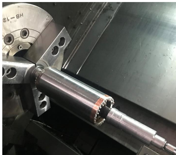
Figure 6.10 Rotor being ground and balanced in longitudinal turning station
