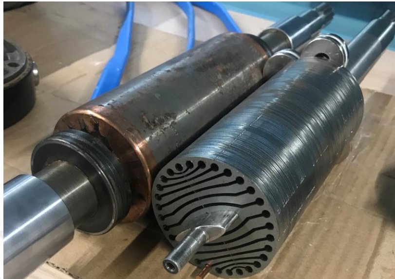
Figure 6.7 Stacked rotor laminations onto the oval shaft
