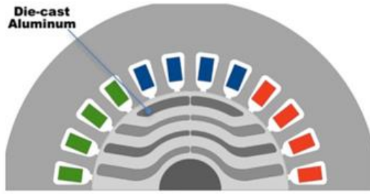
Figure 2.9 Cross section of the motor [39]
