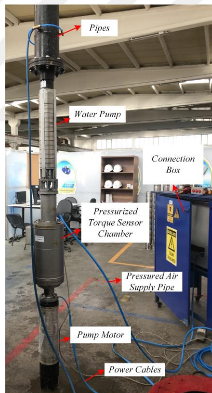
Figure 6.15 Motor under test, torque sensor, and pump assembly
