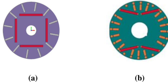
Figure 2.2 (a) The proposed motor with axial rotor slots [20], (b) V-shaped magnet with less active material [3,21]
