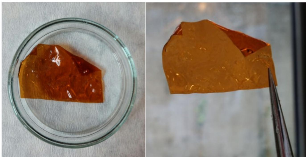
Figure 4.2.4.1 Photo of acid doped mixed matrix membrane
