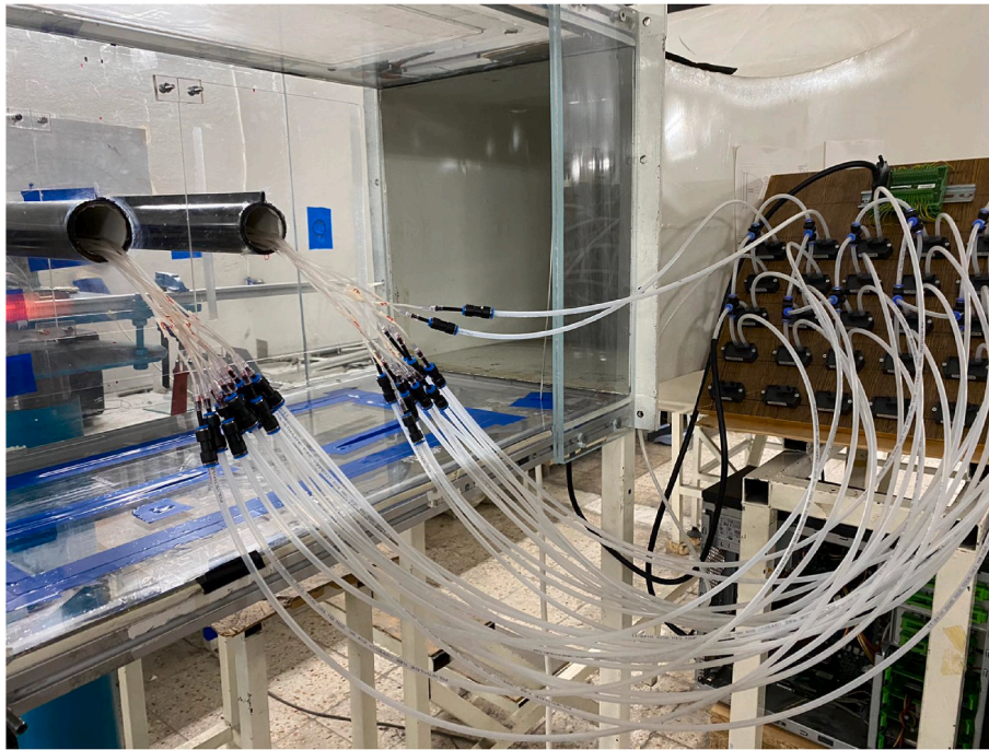
Fig. 9. Pressure measurement test setup.
