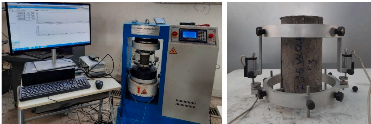
Fig. 2. Experimental set up for compressive strength test.
