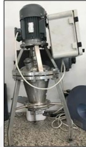
Fig. 1. High-speed paddle mixer.
