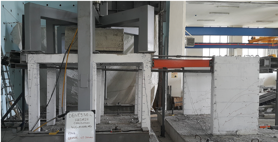
Figure 9. The strengthened system in the 40 th push cycle in the fourth test.
