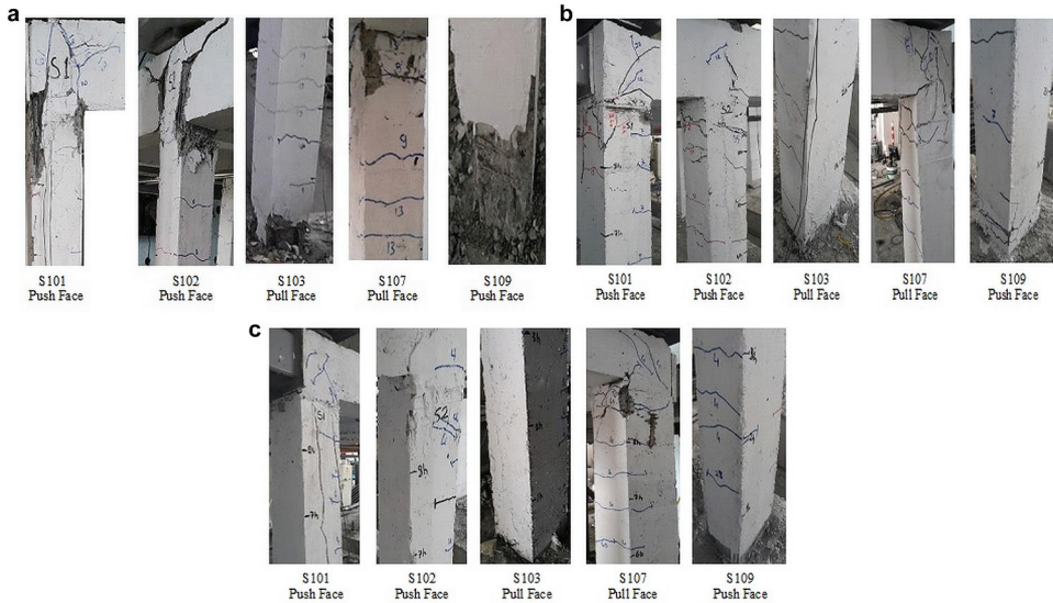
Figure 10. (a) Damage appeared in some columns of the reference frame at the end of the test. (b) Damage appeared in some columns of the strengthened damaged test frame at the end of the test. (c) Damage appeared in some columns of the strengthened undamaged frame at the end of the test.
