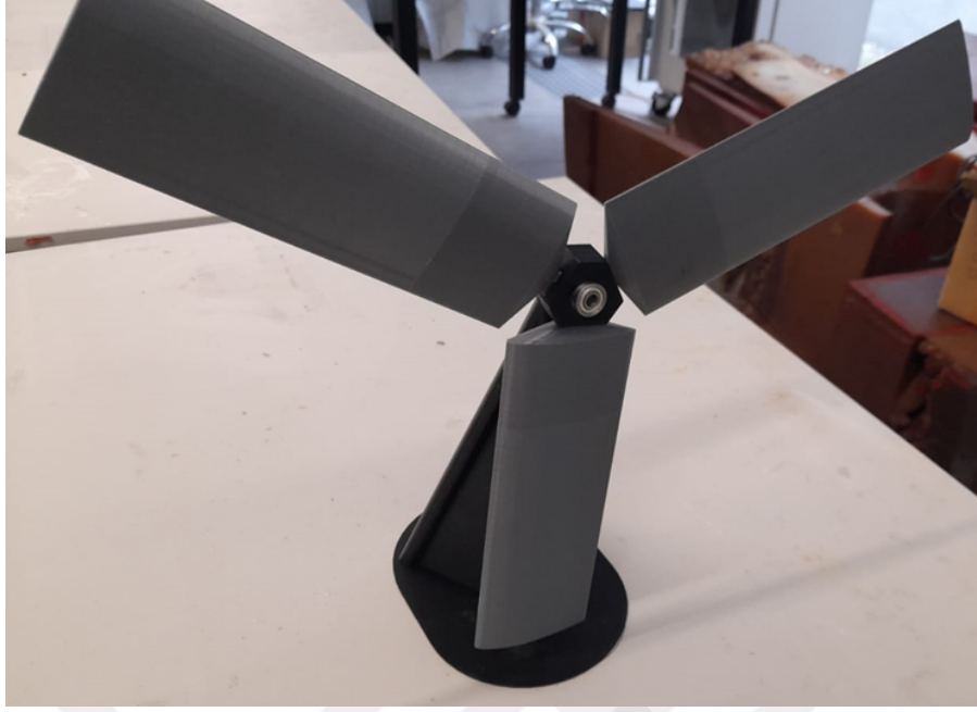
Figure 3. 11 Sample wind turbine produced for wind tunnel tests
