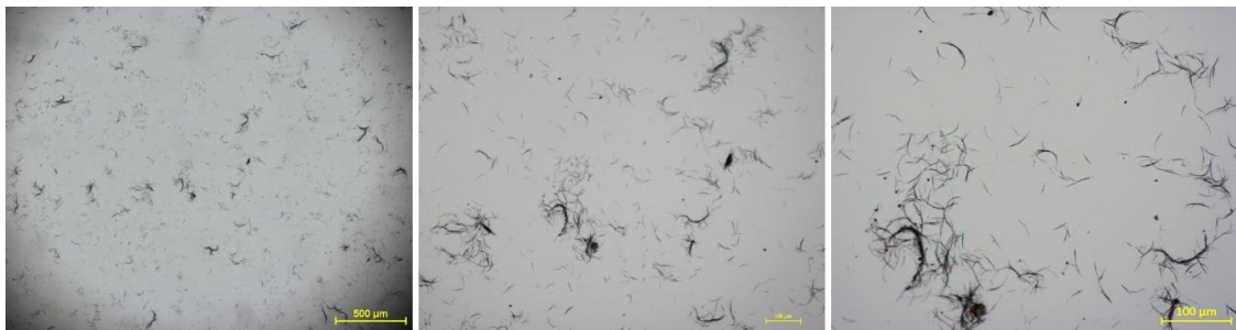
Figure 3. 37: Optical Microscopy Images of AgNWs coated glass, without laser light application
