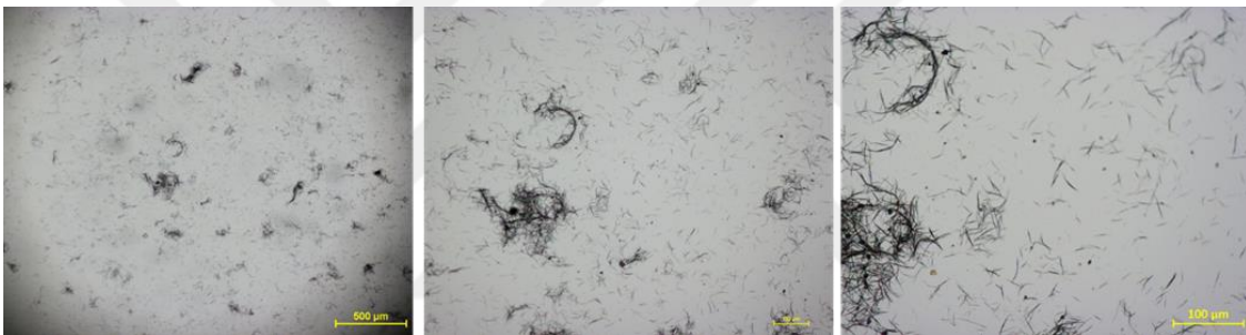
Figure 3. 39: Optical Microscopy Images of AgNWs coated glass, after application of focused blue laser light for 30 min
