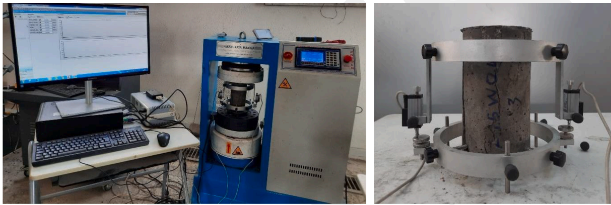
Fig. 2. Experimental set up for compressive strength test.
