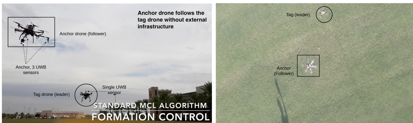
Fig. 2 Front (left) and top (right) views of an outdoor experiment of a drone with three UWB sensors (hexacopter) estimate the relative position toward another drone (quadcopter) with a single UWB sensor by using the three distance measurements. The estimation signal is fed
